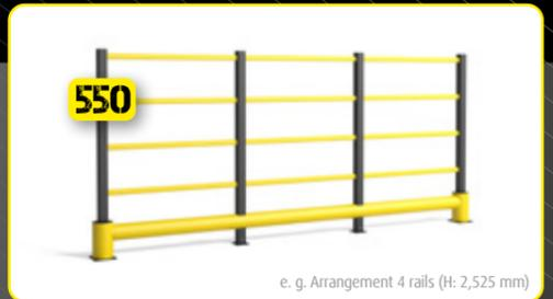
► The TB 400 GRILL with single tube protects people against the impact of forklifts and falling goods. Depending on the size of the (stacked) goods, one can opt for an arrangement with a centre distance between the rails of 275 mm or 550 mm (max. height: 3,075 mm).
